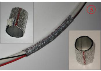
You can then proceed with the external bonding. The result of a proper bonding is as shown in Figure 5. The inside line (blue in the example) is covered and the external line (red in the example) is visible.
