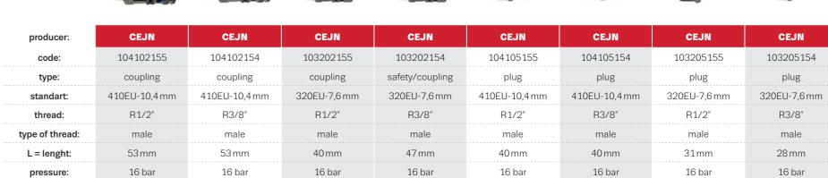
Serie 320 - working pressure 16 bar, min. burst pressure 140 bar, flow capacity 21001 / min Serie 410 - working pressure 16 bar, min. burst pressure 140 bar, flow capacity 39001 / min
