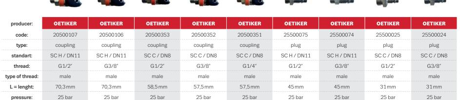
Serie DN8 - working pressure 25 bar, disconnection pressure 15 bar Serie DN11 - working pressure 25 bar, disconnection pressure 15 bar
