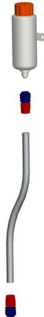
Figure 15: Oil breather catch tank
