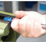
5. Complete the assembly using the correct size spanner and tighten until there is a maximum gap between socket and fitting of 1mm. **Under no circumstances undo the fitting to adjust the alignment.** 6. Pressure test the assembly to 2 x maximum working pressure, clean, inspect and plug ends for storage.
