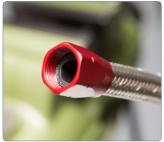
3. Lightly lubricate the fitting threads and the inside of the hose with clean lubricating oil. Hold the fitting horizontally in a vise and thread the hose and socket on by hand as far as possible - taking care not to cross the threads.
